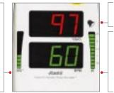
The Alarm Status Indicator flashes when an alarm condition is present.
